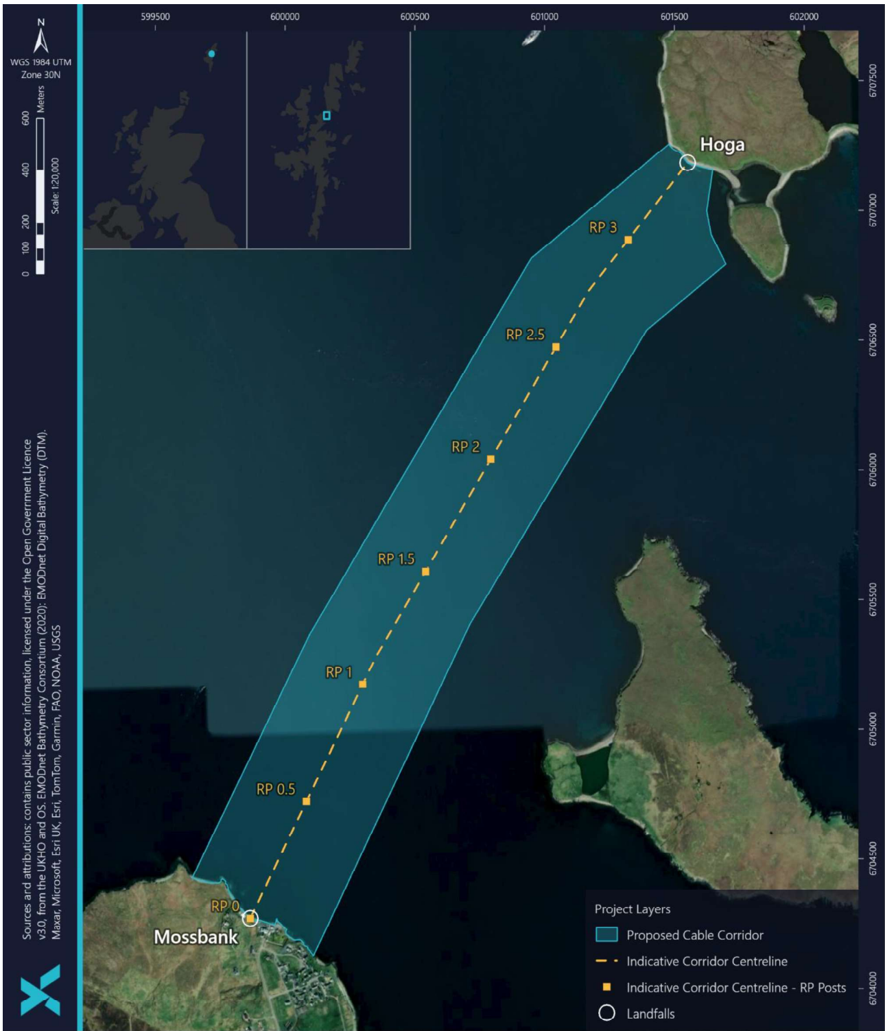
Figure 1-2 The Mainland Shetland (Mossbank) – Yell (Hoga) Proposed Cable Corridor (Note: indicative corridor centreline does not depict proposed cable route but is provided for spatial referencing within the proposed cable corridor, in combination with the Reference Points (RPs)).
