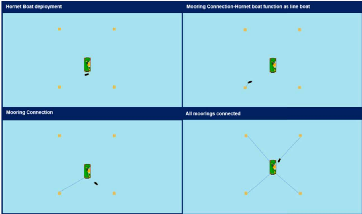
Figure 4-4 Diagram showing a 4- Point Mooring design
