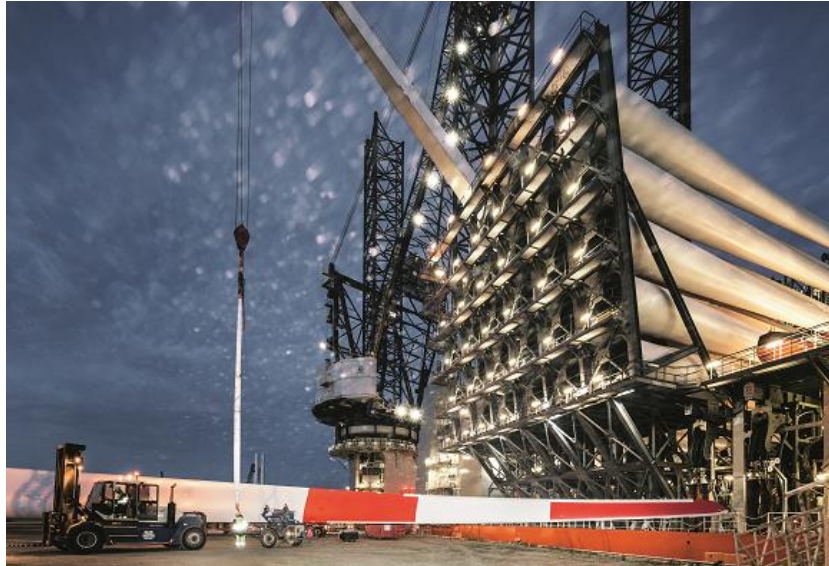
Figure 5.20 - Example of jack up vessel being loaded with wind turbine components
