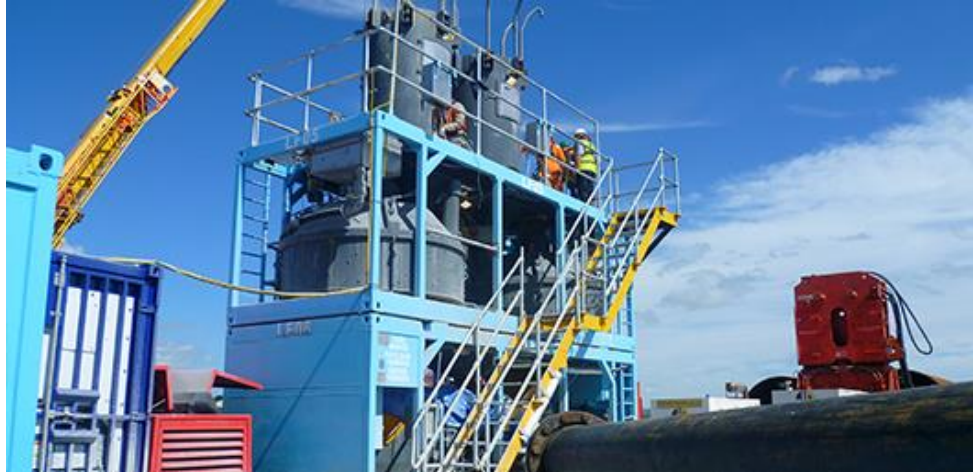
Figure 5.12 - Example of grouting spread set up on a HLV
