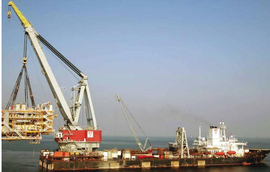
Figure 5.26 – SHL vessel performing heavy lift of a conventional offshore substation platform topside
