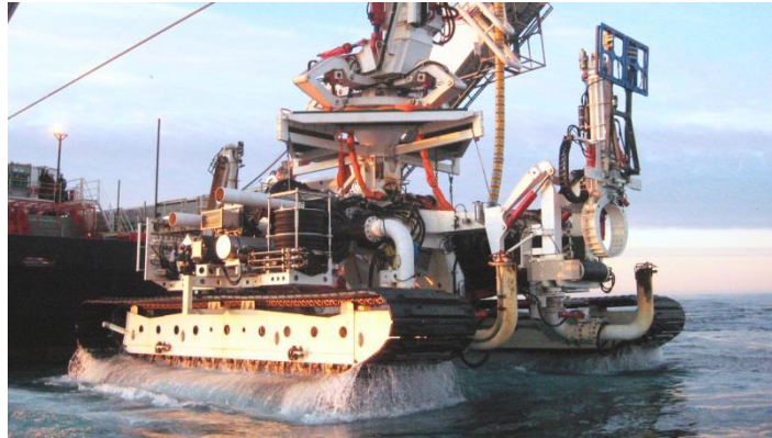
Figure 9.8 - Examples of seabed water jetting cable trenching tools that may be used for inter-array cable installation
