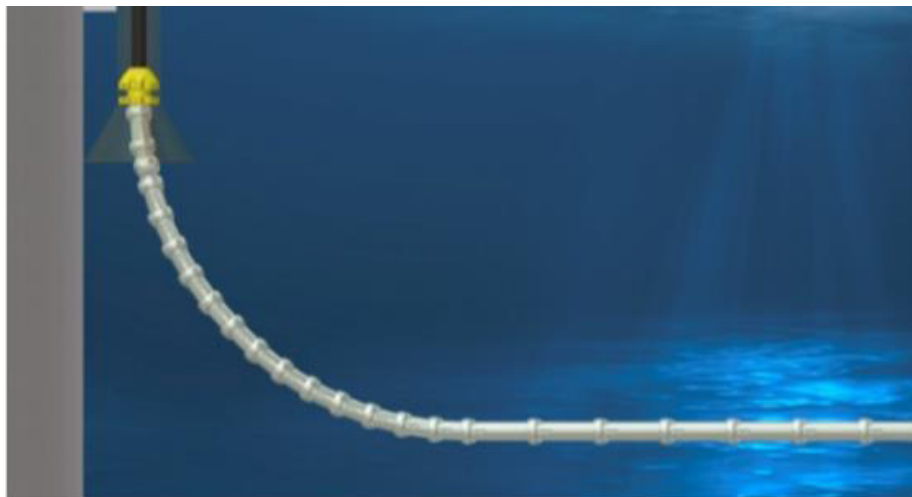
Figure 9.9 - Example of cable protection system at OTM or WTG J-tube
