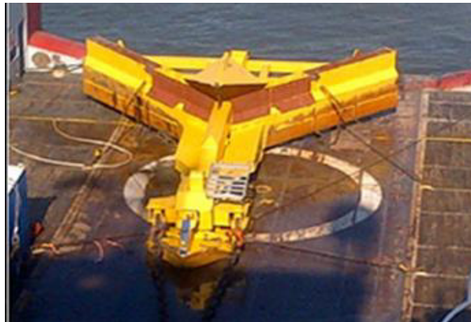
Figure 9.2. SCAR plough configured for boulder clearance operations
