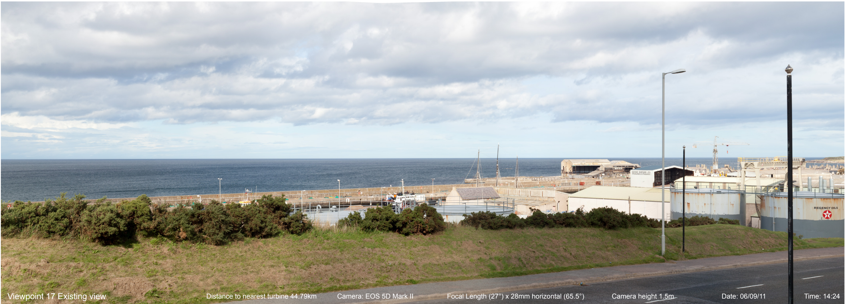
Viewpoint 17 Wireline overlay - Proposed Wind Farm Blade Tip: 280m Rotor Diameter: 230m No. of Turbines: 100
