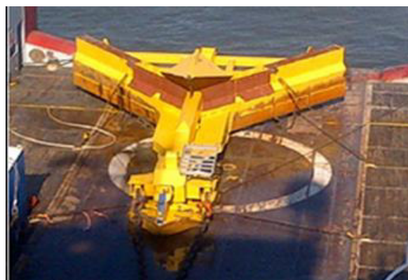
Figure 5.3 - SCAR plough configured for boulder clearance operations.
