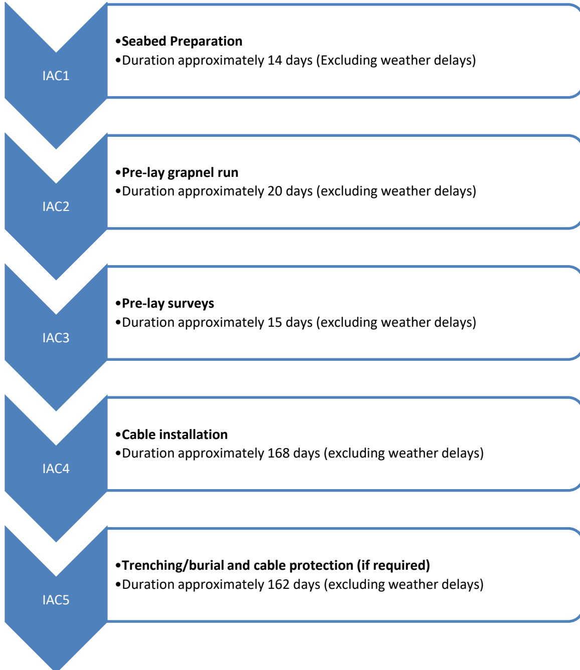
Figure 5.12 Inter-array Cable Installation Sequence
