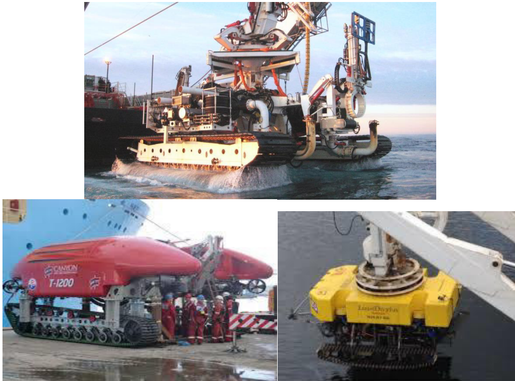
Figure 5.19 – Examples of seabed water jetting cable trenching tools and cable plough that may be used for inter-array cable installation
