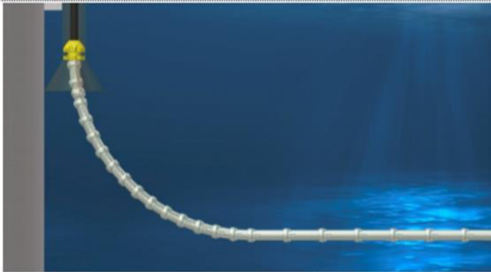
Figure 9.8 - Example of cable protection system at OTM J-tube
