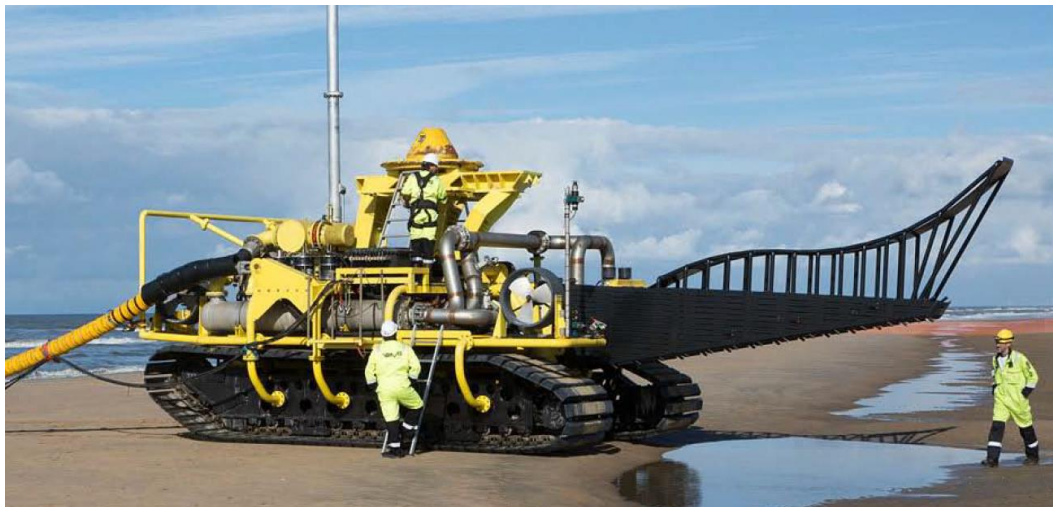
Figure 16 Examples of seabed cable trenching tools (cutting and jetting)
