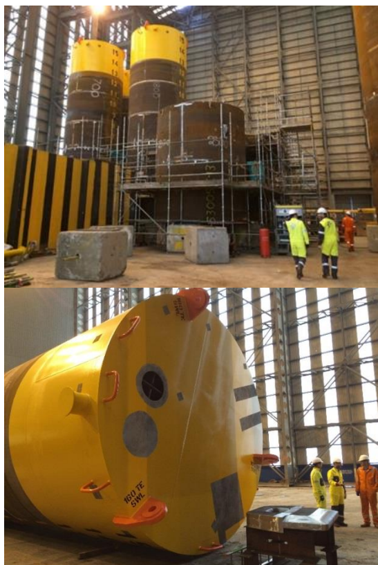
Figure 2.3. Pictures and drawing of suction anchors
