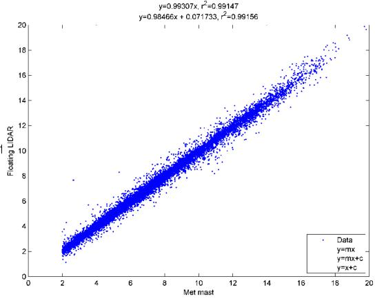
Horizontal Wind Speed (m/s) at 90m LIDAR Time Offset = 00:10:00
