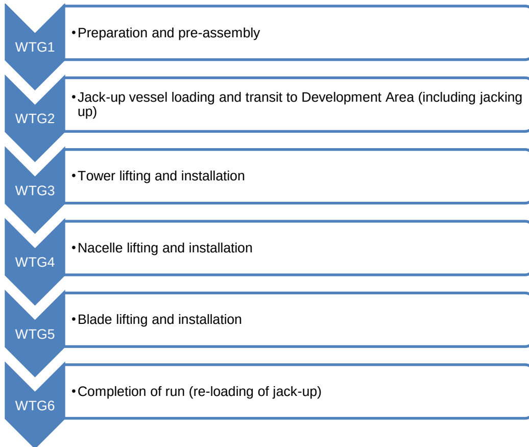
Figure 12 WTG Installation Sequence
