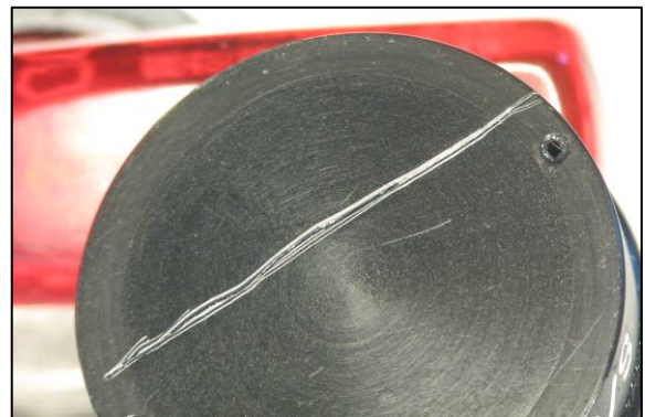
Severely damaged surface still measuring well. The scratch is 0.3 mm wide and 0.2 mm deep.
