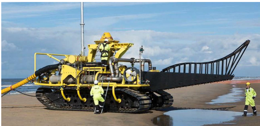
Figure 12 Examples of seabed cable trenching tools (cutting and jetting)
