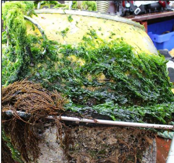
Fouling after fourteen weeks at sea.
