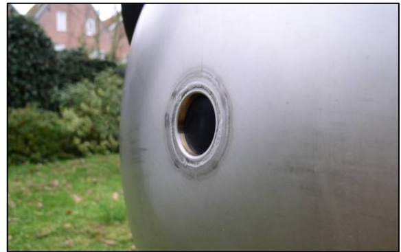
Recessed transducer in the hull.
