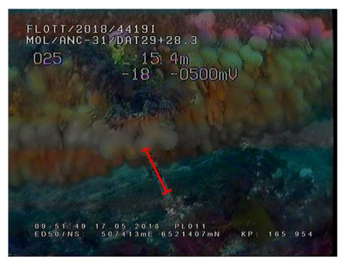
**Rock Anchor Point 41:** At a depth of approximately 16 m and 970 m east from the South Ronaldsay Landfall a scour of approx. 300 mm has been identified. It is deemed appropriate to adequately support the pipeline and the rock anchor with grout bags/mattresses.
