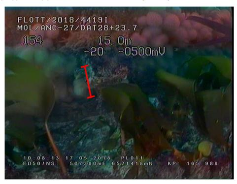
**Rock Anchor Point 31:** Located at 870 m east from the South Ronaldsay Landfall a scour of approx. 300 mm has been identified in multiple inspections as shown below. It is deemed appropriate to adequately support the pipeline and the rock anchor with grout bags/mattresses.
