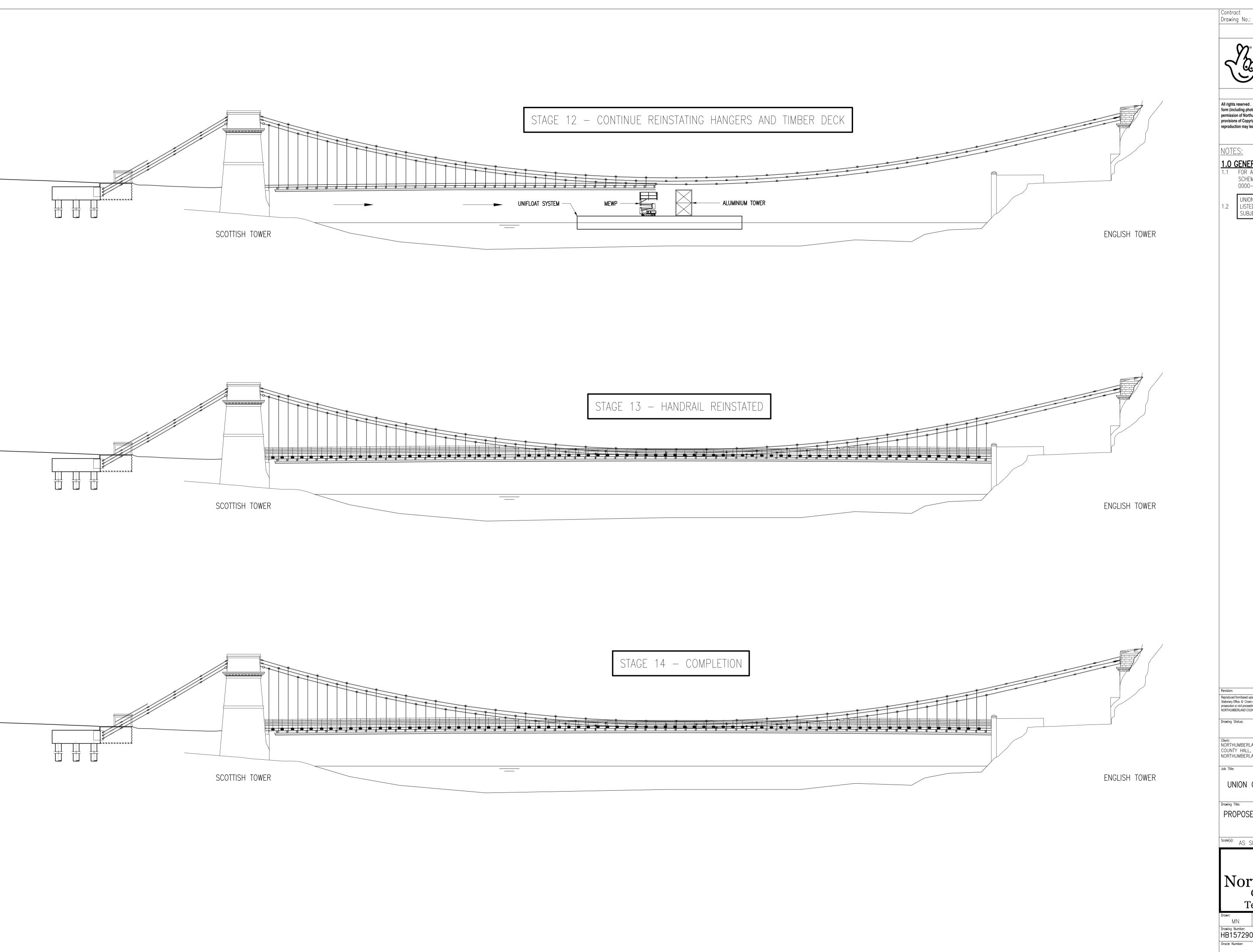
File Path: S:\Highways\PROJECT\15\HB15 Bridges LTP\HB157290 — Union Chain Bridge\Drawings\Working\0000 SERIES DRGS\HB157290—B-C02-TBT-02-0053 Proposed Reconstruction Sheet 4 of 4
