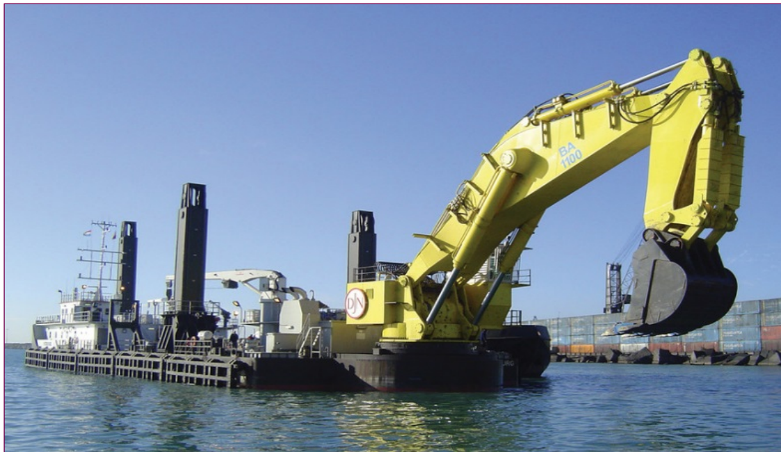
Figure 2.7: Typical Backhoe Dredger
