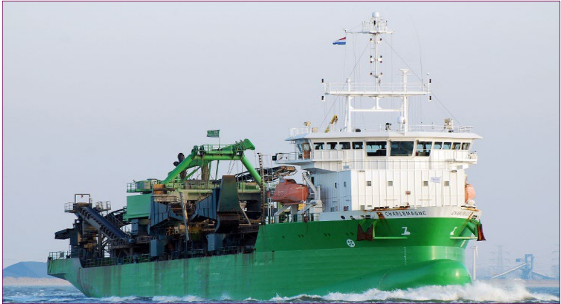
Figure 2.8: Typical Trailing Suction Hopper Dredger
