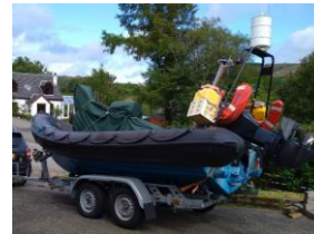
Figure 6: Fast workboat Rigid Hull Inflatable Boat (RHIB) or hard boat 8m – 10m; speed <20 knots
