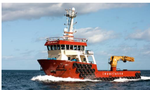
Figure 3: Multicat Vessel Specialised flat-bed mooring vessel ~28m x 10m; speed <12 knots
