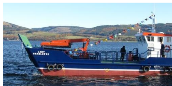
Figure 4: Workboat vessel Versatile landing craft style vessel ~18m x 5m; speed <8 knots
