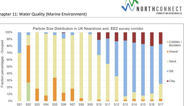
Figure 11.2 Particle Size Distribution from the UK Coast to the UK EEZ limit (MMT, 2018).
