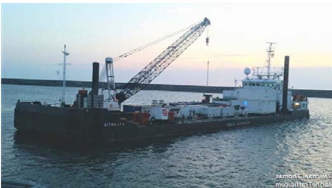
Figure 5-1 Rock Placement Vessel Tideway Atlantis
