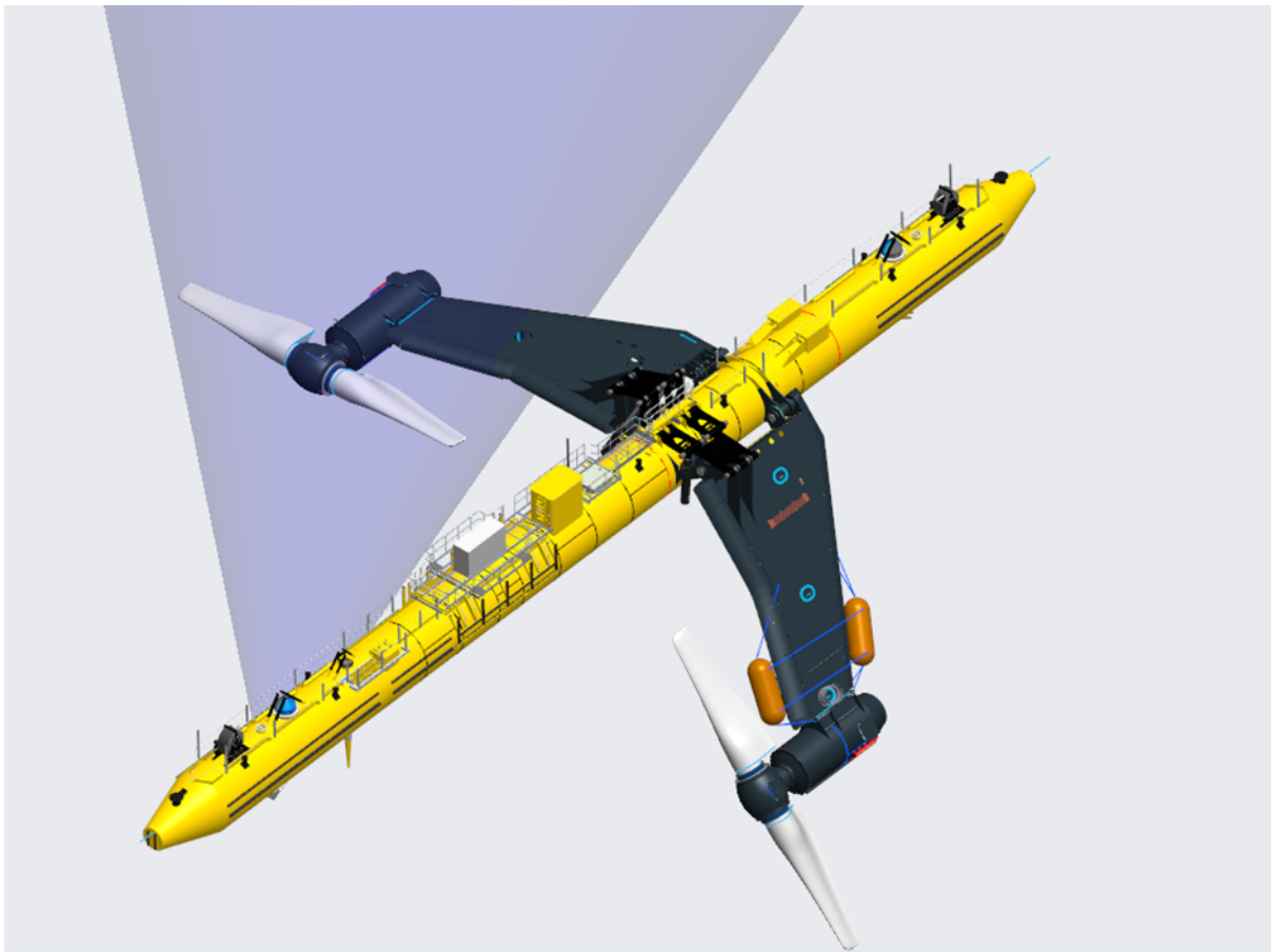
Figure 7. FORWARD2030 sonar placement for O2
