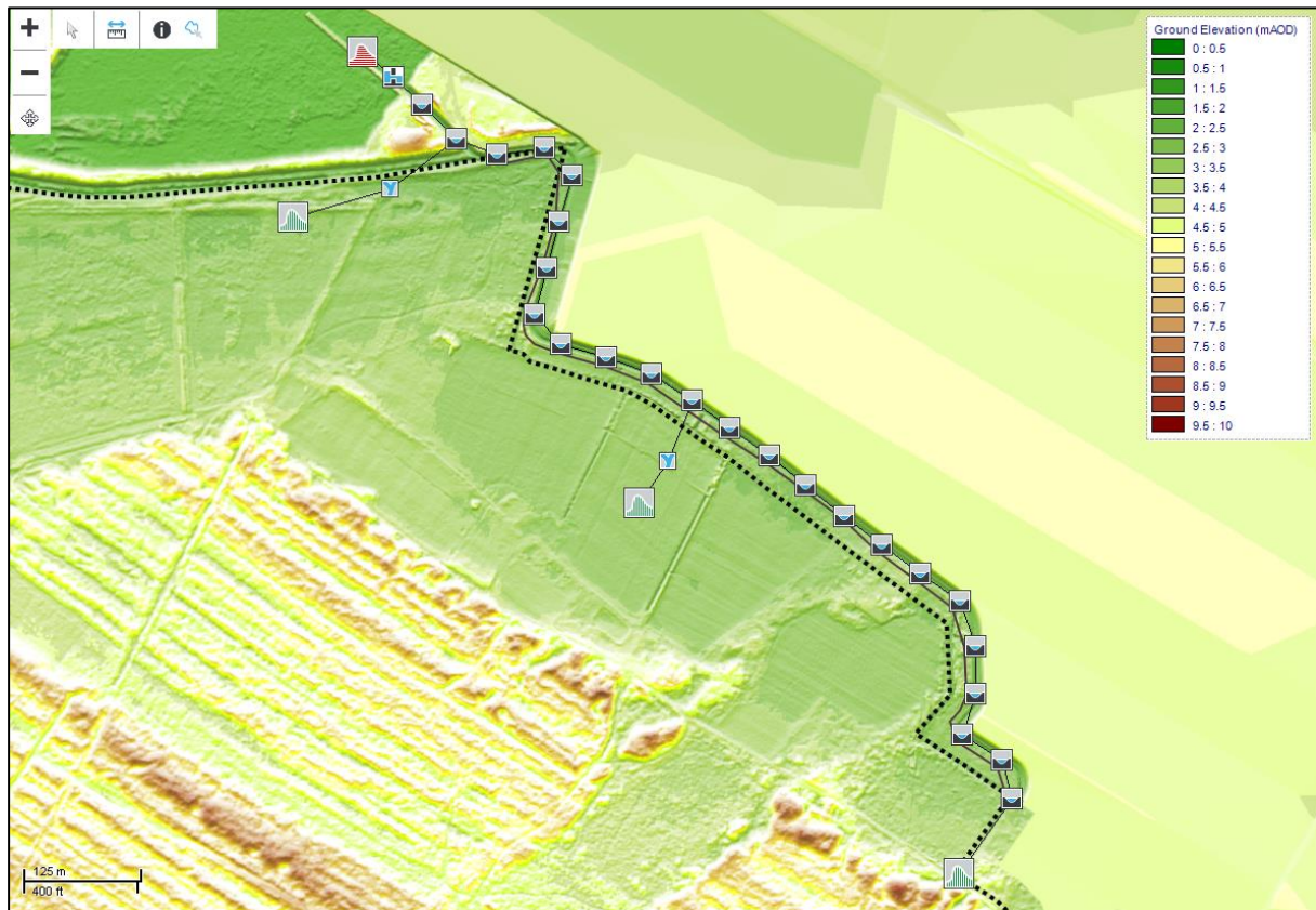
Figure 6.9: Western Watercourse 1D model schematic, with LiDAR-based ground elevations (external to site) and proposed platform elevations (within the site)
