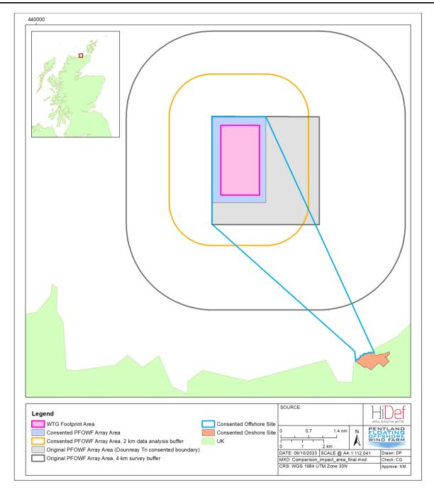
Figure I PFOWF Variation Application proposal, showing the revised array area (the WTG Footprint Area) in pink
