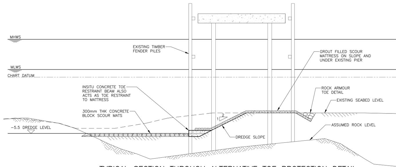
TYPICAL SECTION THROUGH ALTERNATIVE TOE PROTECTION DETAIL
