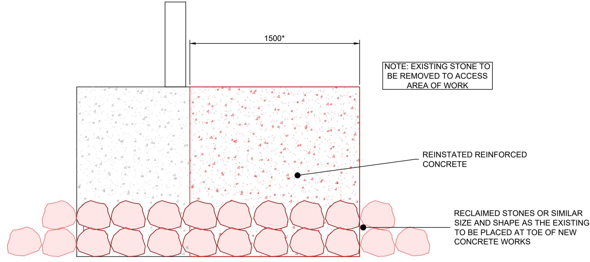
PROPOSED REPAIR No. 3 END ELEVATION
