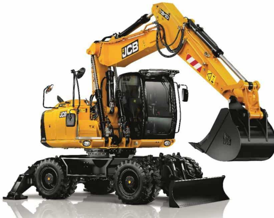
Figure 6 – Excavator JCB JS160
