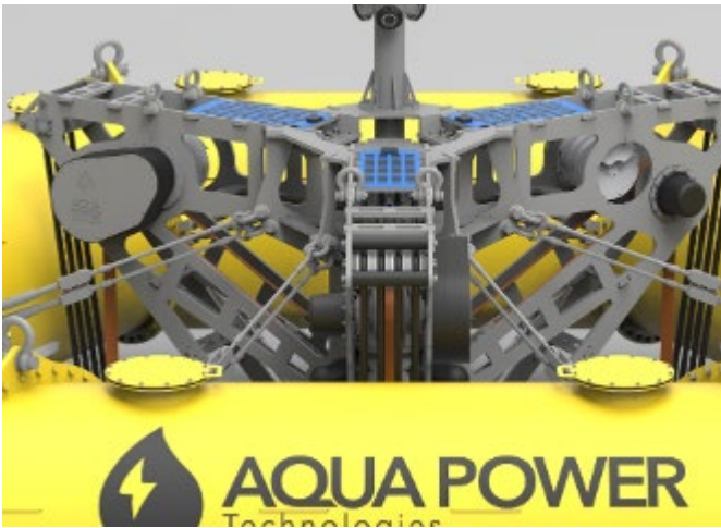
Figure 10 Introduction of belt driven PTO in TriWave.
