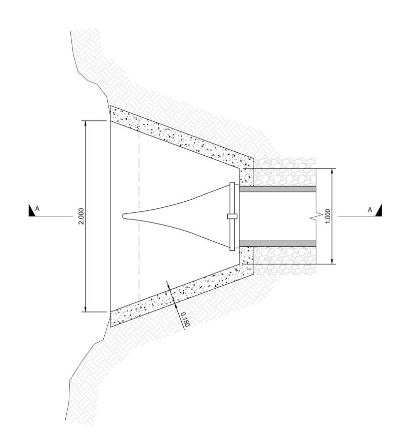
Detail: Plan on Outfall Headwall and TideFlex Valve
