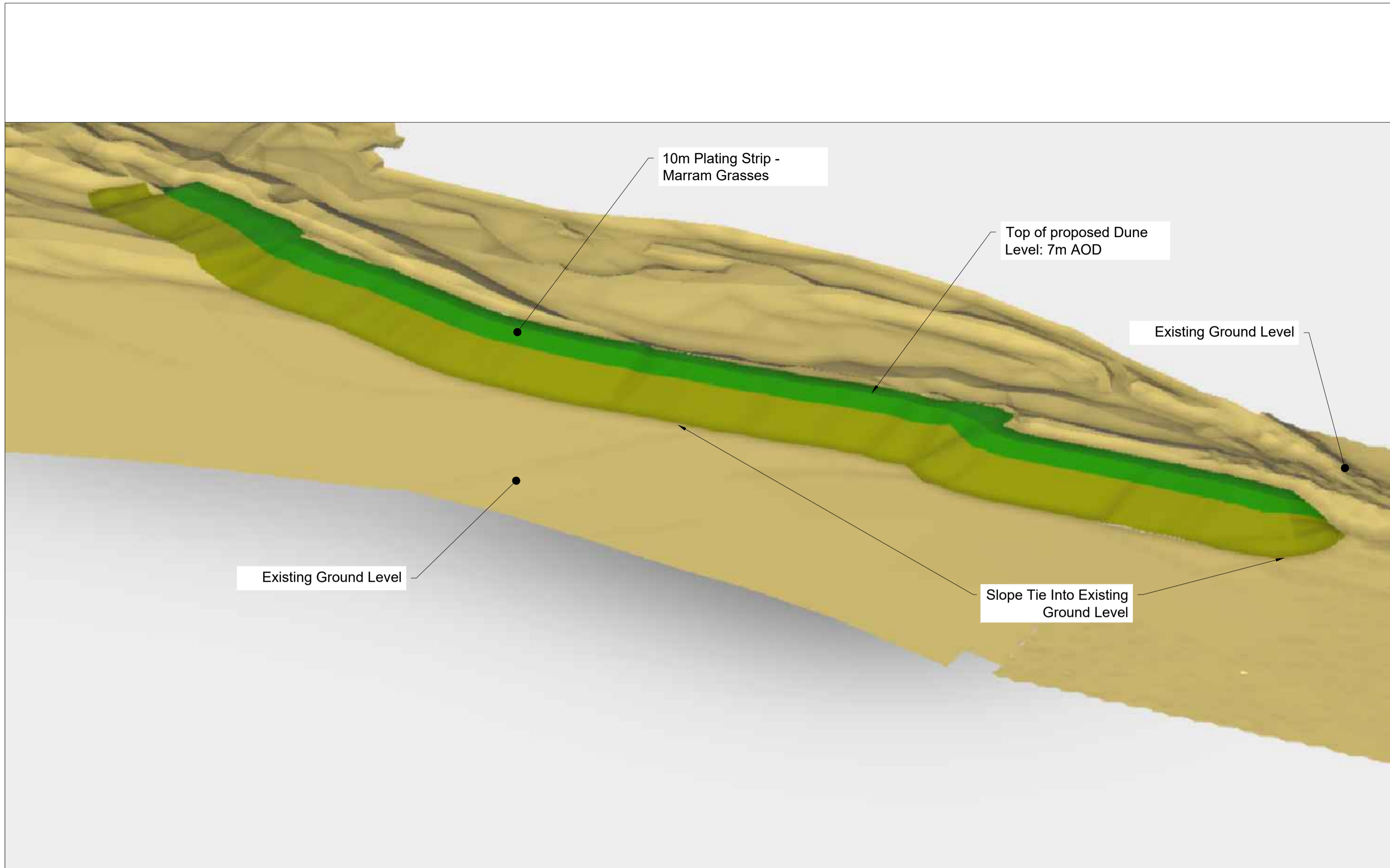
IMAGE 1 PROPOSED MODEL - GENERAL ARRANGEMENT ISOMETRIC VIEW N.T.S
