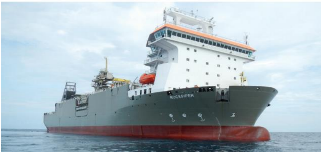
Figure 4-2: An example of a typical subsea rock installation vessel
