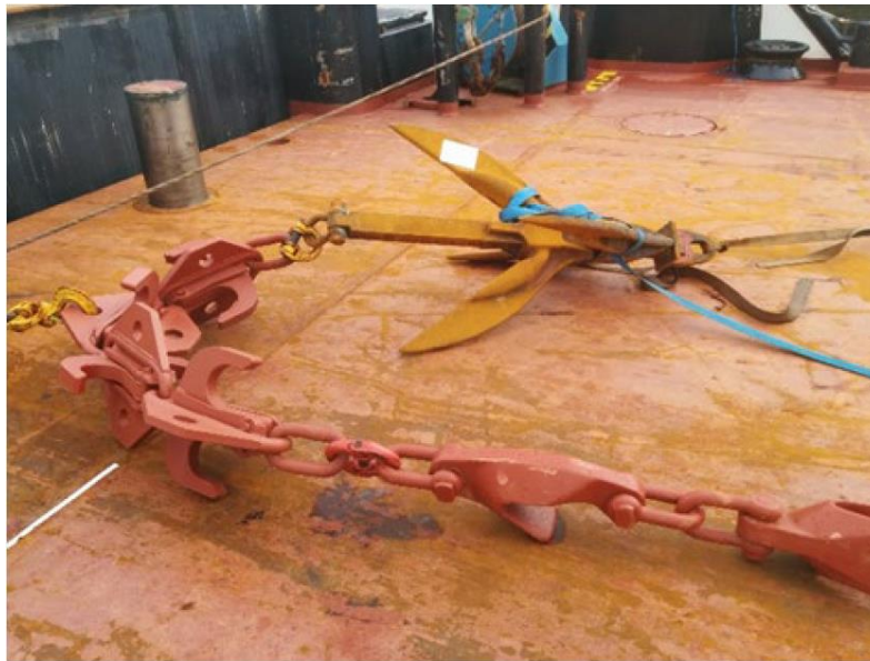
Figure 4-12: Example of a typical PLGR train on board the vessel.
