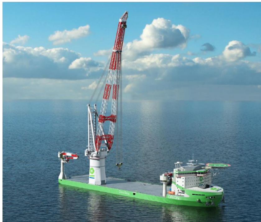
Figure 4-5: Example of a HLV, the 'Orion', which may be used to transport the monopiles from the IDP to the Moray West Site. Such a vessel will be able to install six monopiles per trip.
