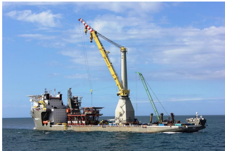
Figure 2-2: Example of pile installation vessels.
