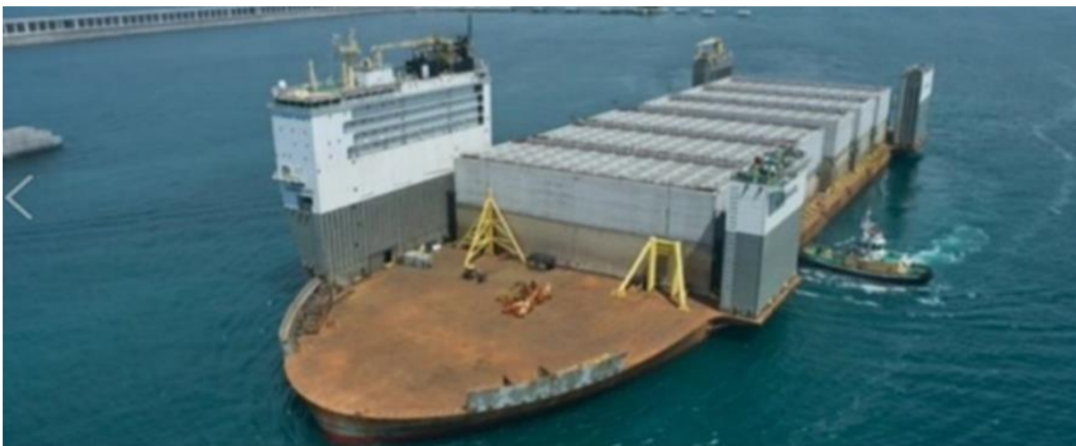
Figure 5-4 Image of caisson loading operation
