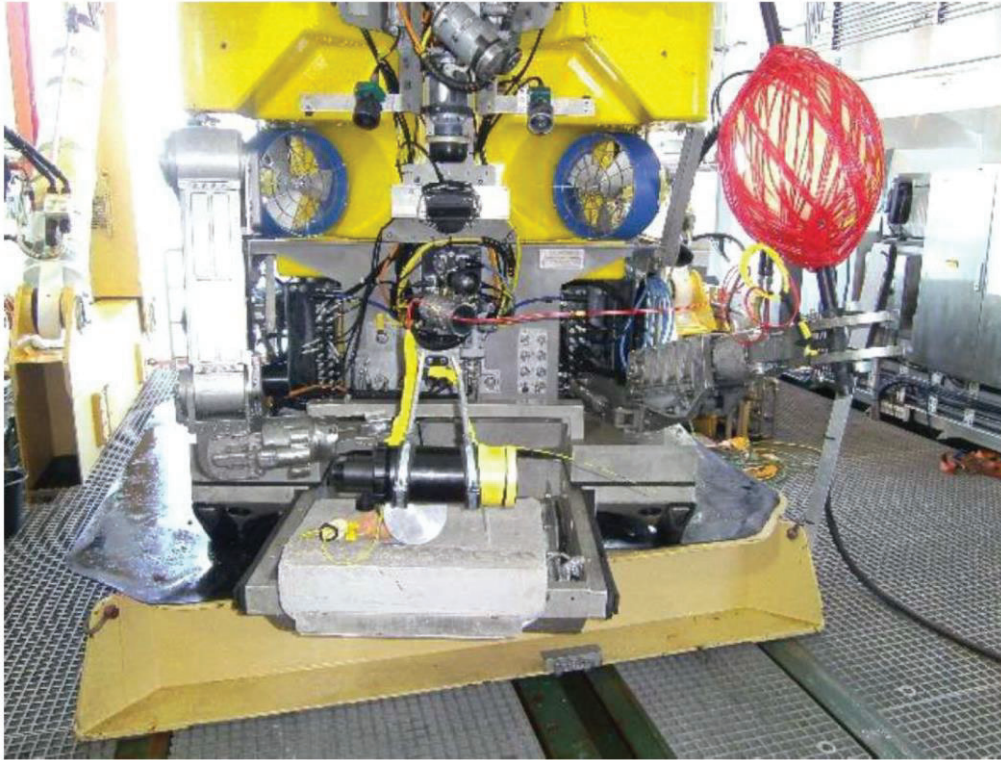
Figure 2-3 Barracuda UXO disposal system
