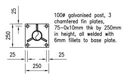
15mm thk base plate with 4.N'. M16 resin anchors, steel grade 8.8, 200mm embedment into existing balustrade concrete foundation.
