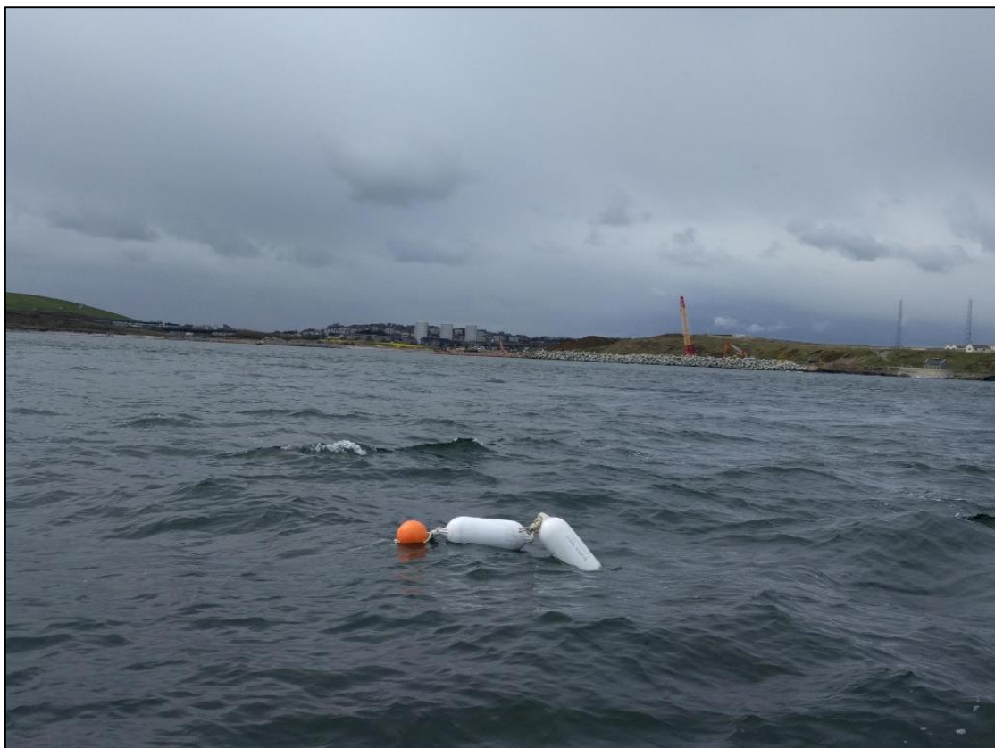
Figure 2: C-POD attached to a mooring line and deployed at AHEP.
