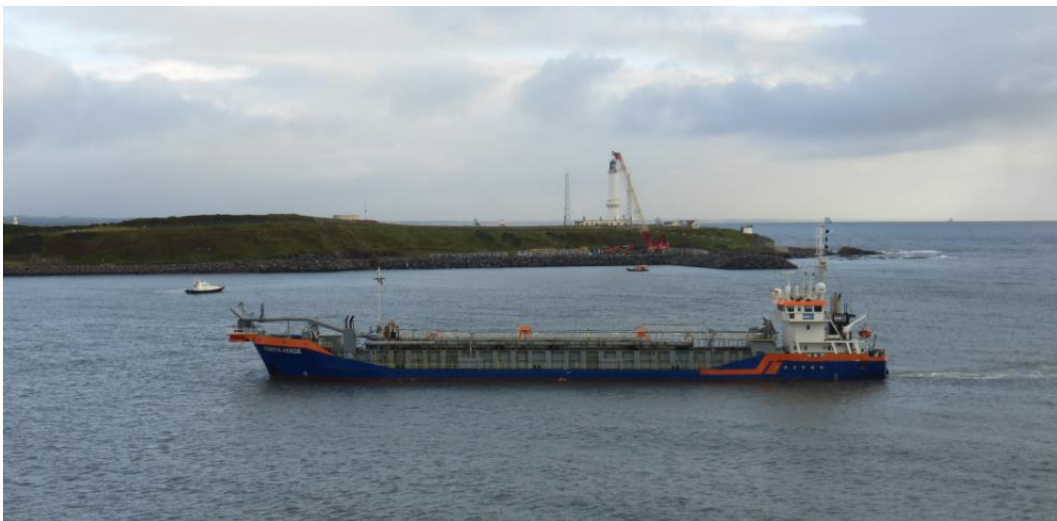
Figure 7.3: Example of a TSHD (Van Oord Costa Verde)
