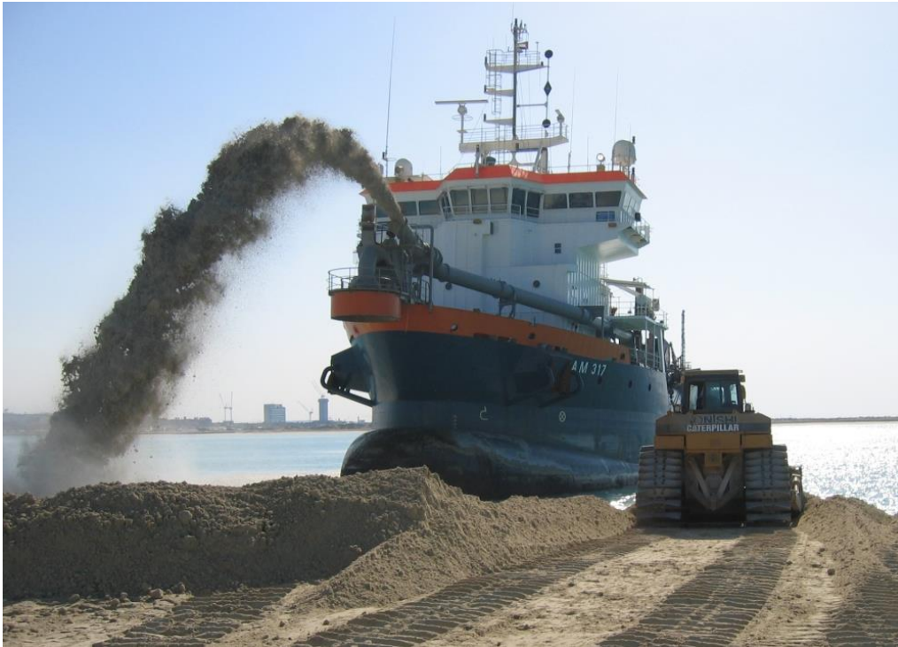
Figure 7.6: Pumping ashore via rainbowing (Van Oord HAM317).
