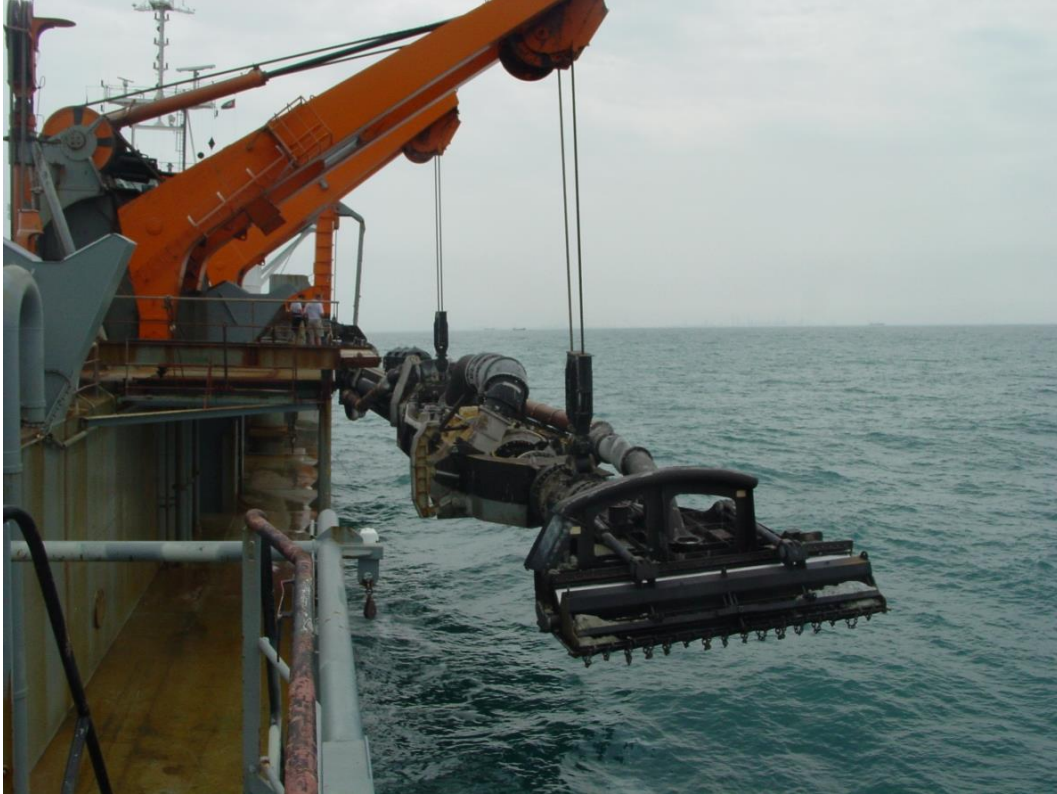
Figure 7.4: TSHD draghead (Van Oord Volvox Terranova)
