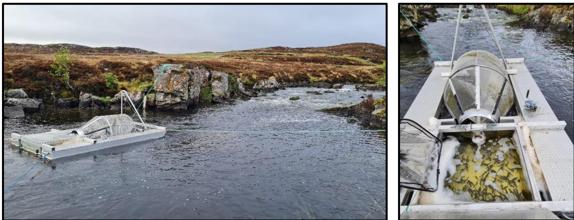
Figure 4 Rotary screw trap deployed to catch out-migrating smolts for tagging in the lower River Grimersta
