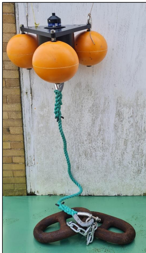
Figure 2 Configuration of an Acoustic Receiver (AR) fixed within the top plate of the Acoustic Retrieval Canister (ARC) with 3 x 11" orange trawl floats on each corner. The AR and ARC are attached to a 70 kg anchor (consisting of 2 x 35kg chain links) via a polysteel rope strop (3 m) and connection chain. Marine grade high load stainless steel shackles are used on all connections.
