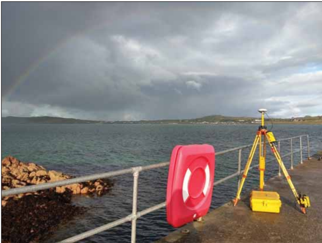
FIGURE 2 - TRIMBLE SPS855 BASE STATION AT BASE 1 LOCATION (FIONNPHORT FERRY PIER)
