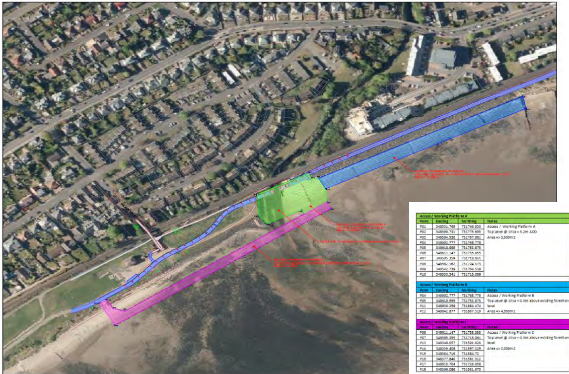
Figure 9: Anticipated Extent of Required Temporary and Permanent Works Below MHWS Over Inter-tidal Area for new bridge construction.
