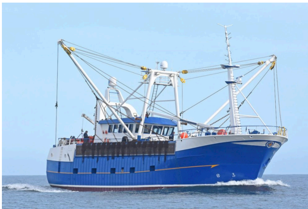
Figure 5.7: Typical scallop dredge vessel (Source: Fishing News)
