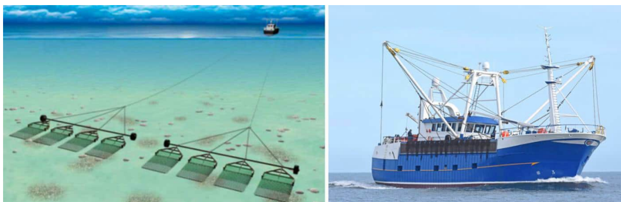
Plate 4.2 Profile of typical scallop dredging gear and vessel (Montgomerie, 2022; Fishing News, 2020)
