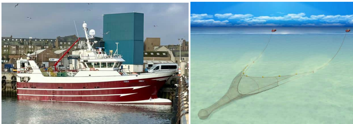
Plate 4.1 Profile of typical demersal otter trawler vessel (NiMa) and pair trawl gear diagram (Montgomery, 2022).
