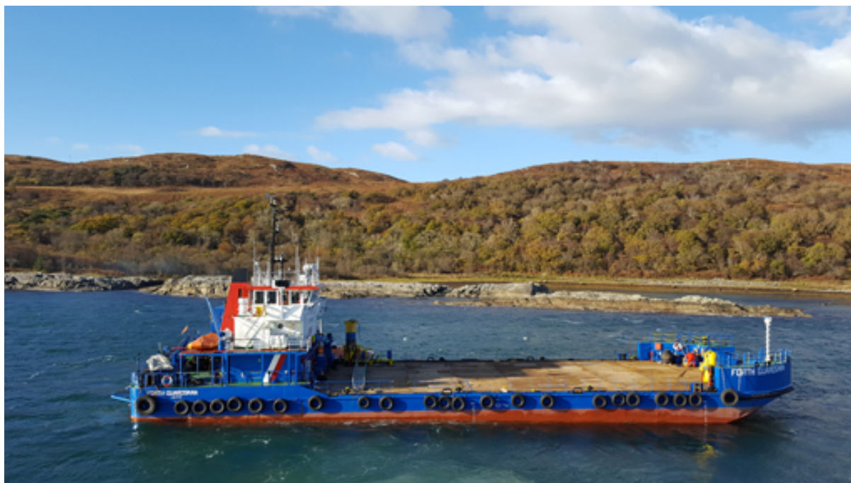
Fig 4 - Forth Guardsman with Spud Legs Deployed (yellow capped piles)
