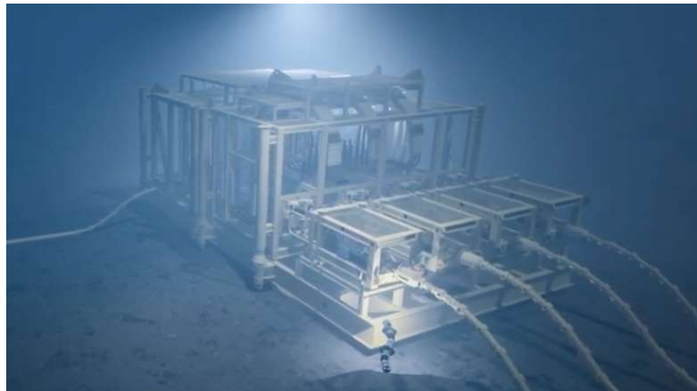
Figure 3-10: Example of a Subsea OEP
