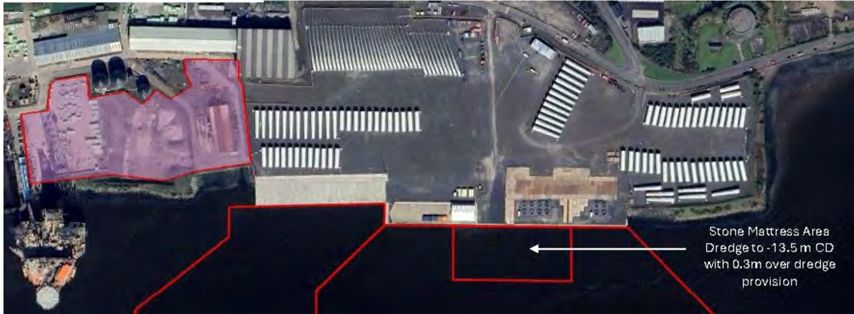
Figure 2-2 Proposed western extension of the laydown area (shaded in pink) of at the Port of Dundee
