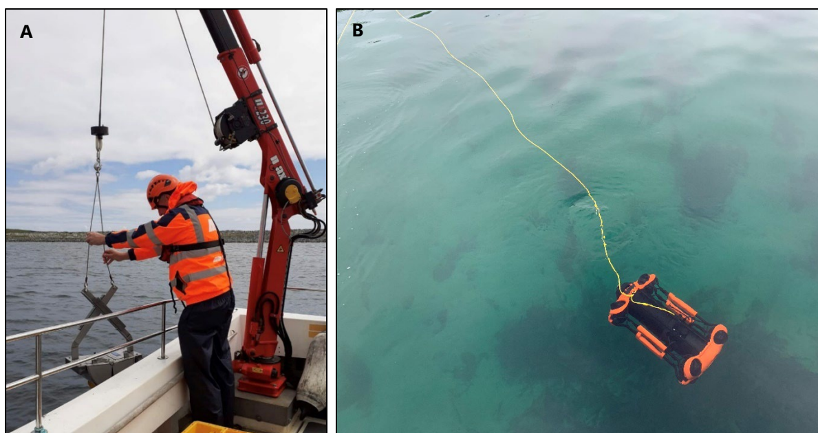
Figure 3. A) Van Veen grab sampling, B) Chasing M2 Pro' Remotely Operated Underwater Vehicle (ROV)
