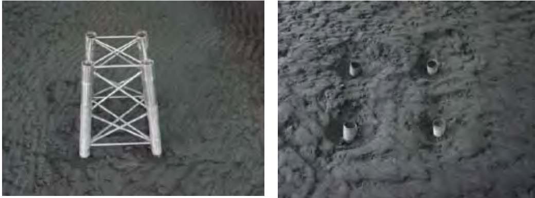
Figure 2.2 Extent of scour observed around the physical model experiments
