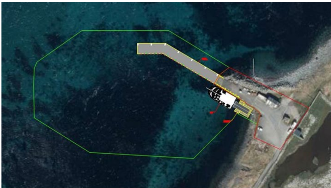
Figure 2. Indicative boundaries of marine works (in green) (1.44 ha) and land based works (in red) (0.21 ha)
