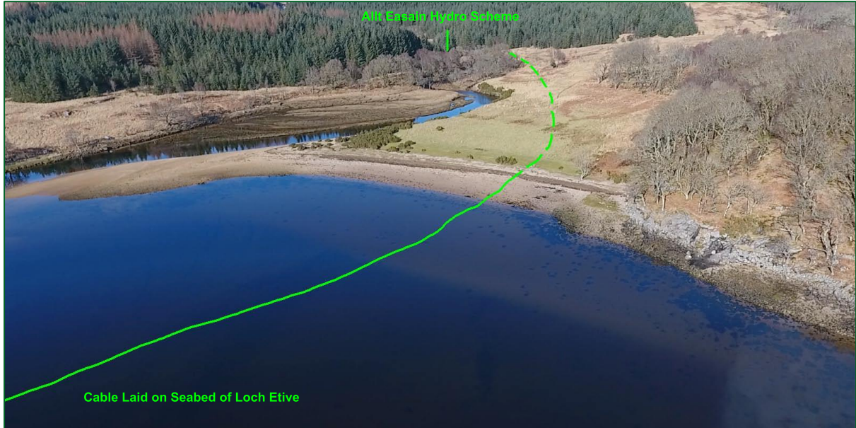
Image 1 – Rubha Bharr Shore End on West Side of Loch Etive. The image was used for the cable licence application, however it demonstrates well the position of the causeway which would be just to the left of the cable, avoiding the small cluster of gorse bushes immediately adjacent to the cable line
