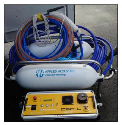
Figure 4 - Applied Acoustics boomer system utilised for the sub-bottom profiler surveys
