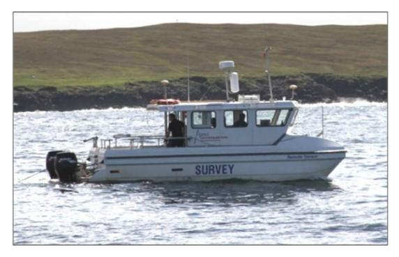
Figure 35 - Survey vessel Remote Sensor with multibeam sonar and towed sensors deployed
