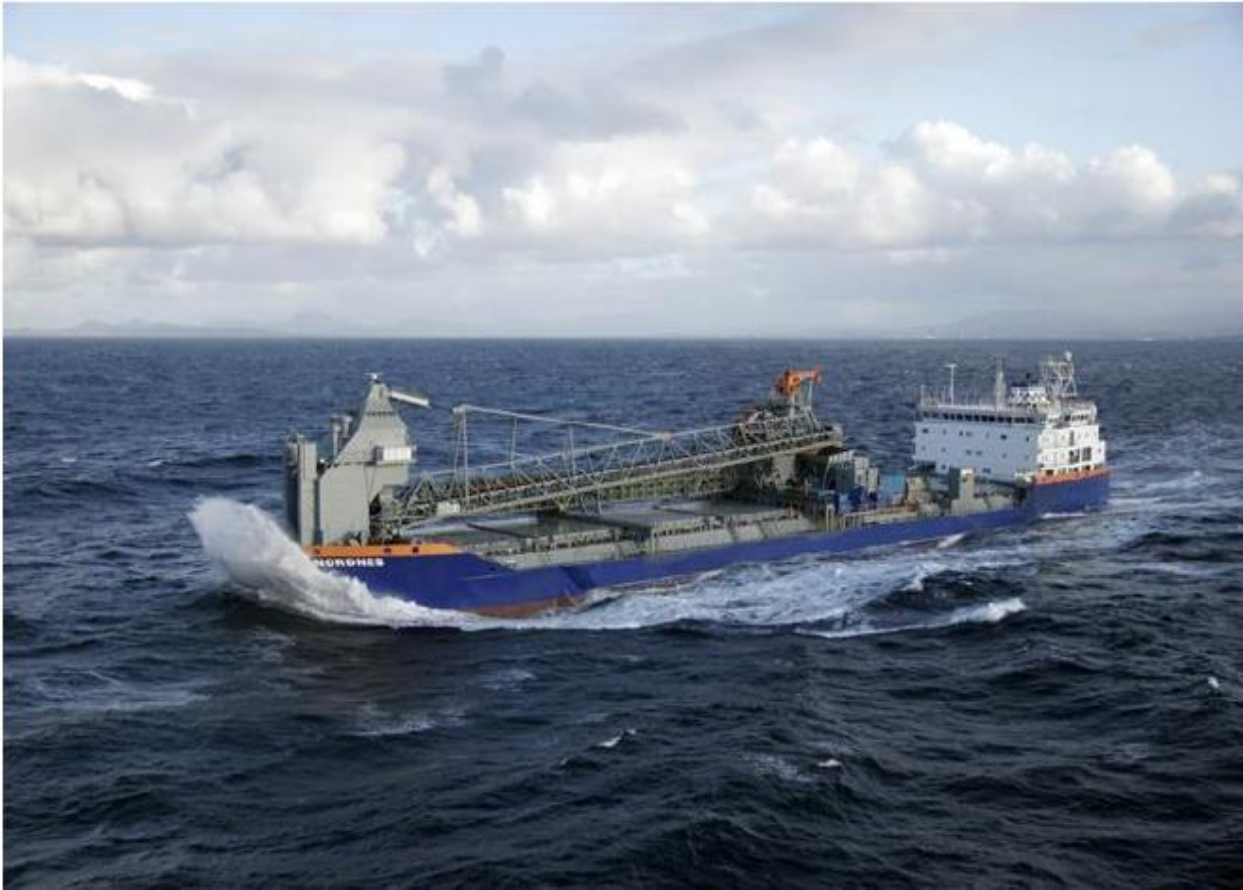
FIGURE 4-7 A TYPICAL FLEXIBLE FALL PIPE VESSEL
