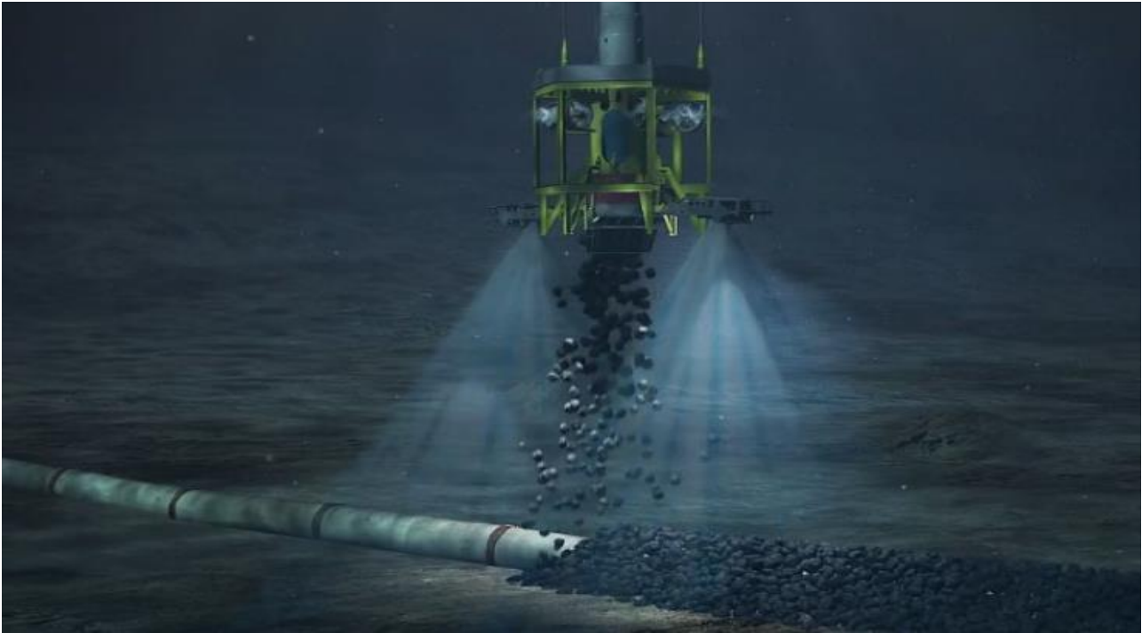
FIGURE 4-6 A REMOTELY OPERATED VEHICLE AT END OF FALL PIPE
