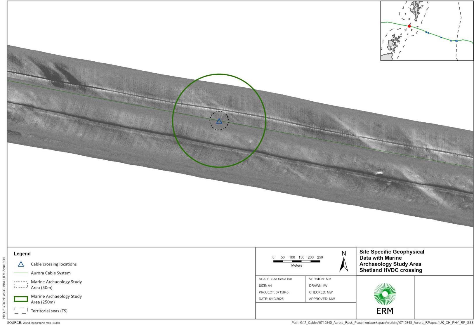
FIGURE E-14 SIDESCAN SONAR AT SHETLAND HVDC ROCK PLACEMENT LOCATION
