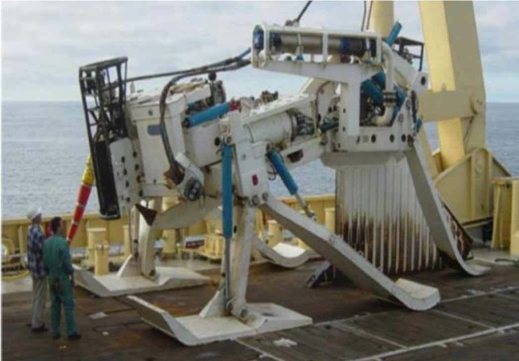
FIGURE 4-8 A SEA PLOUGH READY TO BE DEPLOYED FROM INSTALLATION VESSEL
